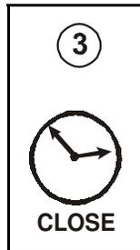
The close run timer establishes the period of time that the actuator motor operates when it receives the command to close an air inlet baffle board or air inlet curtain.
