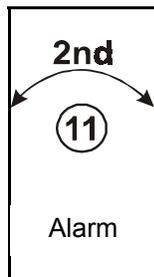
This function establishes the temperature / pressure **difference** above the main set point that the room can reach before a high temperature / pressure alarm is signalled. When a high temperature / pressure alarm occurs the alarm relay is activated and the alarm LED lights on the CPS-1.
