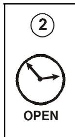
The open run timer establishes the period of time that the actuator motor operates when it receives the command to open an air inlet baffle board or air inlet curtain.
