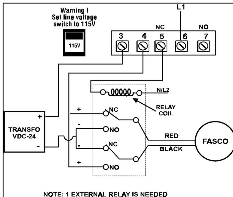
Fig 4a Two actuators connected on the same output
