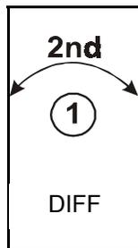
In order to minimize erratic behavior of the actuator motor when the ambient room temperature or static pressure is exactly at the main set point, the differential setting separates this ON / OFF threshold into two: one ON threshold and one OFF. This feature greatly reduces equipment wear.
