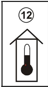
This function displays the ambient room temperature or static pressure of the room.
