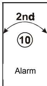
This function establishes the temperature / pressure **difference** below the main set point that the room can reach before a low temperature alarm is signalled. When a low temperature / pressure alarm occurs the alarm relay is activated and the alarm LED lights on the CPS-1.
